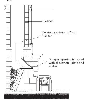
The inside area of the flue liner must not be less than the area of the stove's flue exit, and cannot be more than three times greater than the cross sectional area of the stove's flue exit. If the chimney liner is too large to accommodate the stove, an approved relining system must be installed to resize the flue.
